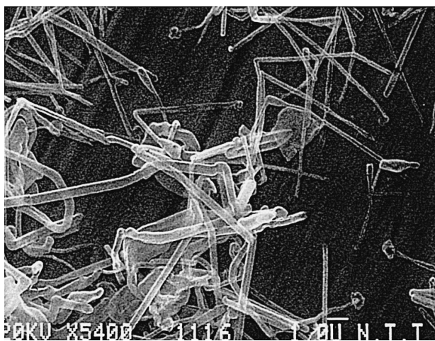
Fig. 1. SEM photograph of lithium deposited in \text{EC}/2\text{MeTHF}/\text{LiAsF}_6 electrolyte at 0.5 \text{ mA}/\text{cm}^2 for 10 min.
